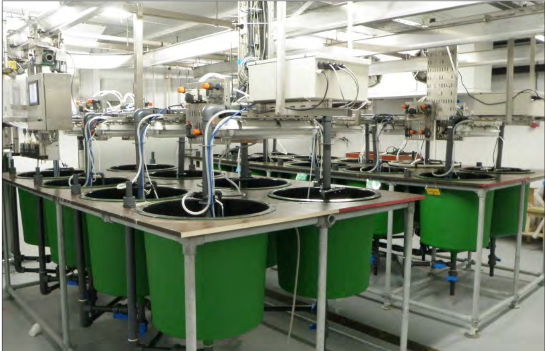
Figure 1. NTNU and SINTEF SeaLab laboratories for start feeding experiments. 18 tanks (160 L) with automatised feeding of live prey (Storvik robot), plankton counter and video surveillance in all tanks. Recirculation or flow-through system. Photo: SINTEF
